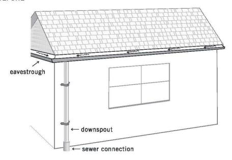
AFTER – eavestrough has been replaced and re-graded to slope towards the new downspout location
