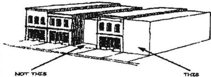
NEW FACADES ARE BUILT FLUSH WITH THE EXISTING STOREFRONTS.
