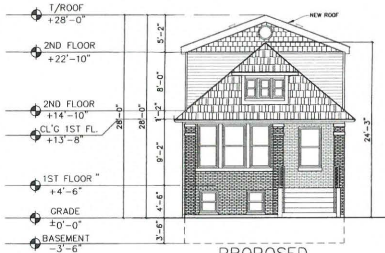
PROPOSED EAST ELEVATION SCALE 1/8" = 1'-0"
